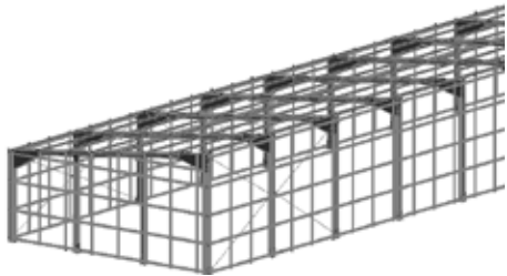
-Sem Platibanda - Fachada Horizontal -Without Parapet - Horizontal Wall Cladding -Sans Prise - Façade Horizontale -Sin Platibanda - Fachada Horizontal
